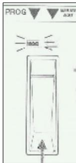
**1** When the power is first turned on, the A5 GUITAR automatically enters into the Program mode. To switch to the Program mode from the Manual Edit mode simply press the Mode Select Switch.
