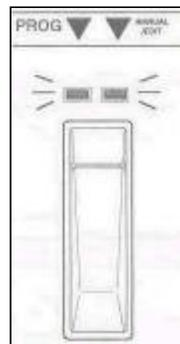
Both Mode LEDs light up for about a second to indicate that the writing operation is completed.
