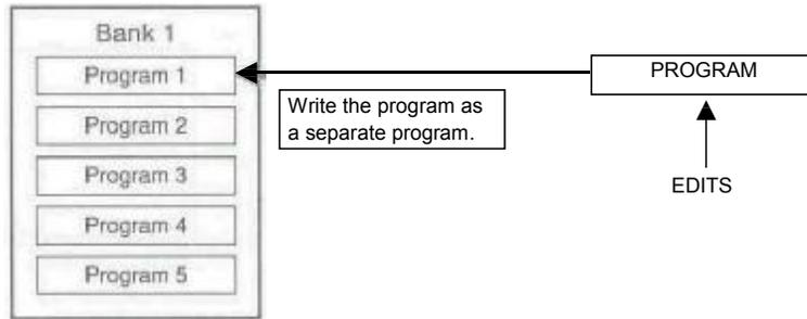
**1** When editing is completed in the Edit mode, press the Write key to save the currently edited program. For example an edited version of METAL 1 (Program number 1 in Bank 2) is saved as a separate program.
