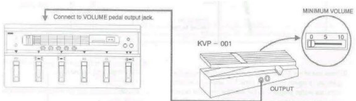
Use the KORG KVP 001 volume pedal. Connect the output jack (OUTPUT) of the KVP 001 into the VOLUME pedal jack (PEDAL) of the A5 GUITAR (Also make sure that the KVP 001 slider has been set to the minimum volume of "0").
