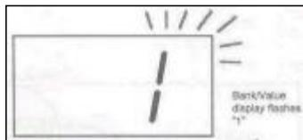
**3** Press the Write key once again. When writing operation is finished both Mode LED's light up for about a second.
