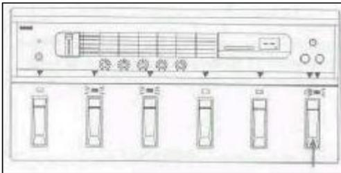
**2.** Enter the Edit mode by pressing the Mode Select Switch. The Mode LEDs, the Value Display and the EFCT/PROG LED s will change to indicate the Edit mode.
