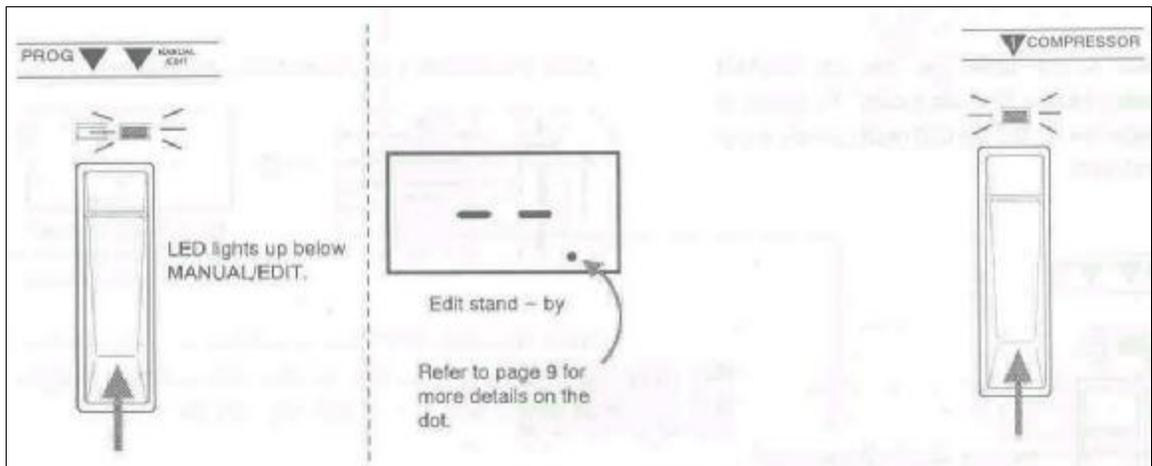
In the Manual/Edit mode, the EFCT/PROG switches (along with the EFCT/PROG LEDs) control ON/OFF of each of the five effects. When entering the Manual/Edit mode the EFCT/PROG LEDs light up to display the effects which are currently turned on. For example the figure below shows that the Manual/Edit mode is selected after selecting METAL 1" in the Program mode.
